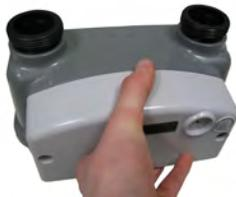
6. Use the screws from the original index to attach the new index to the meter. Tighten the screws by hand with a Phillips or slot head screwdriver to a torque between 6 and 15 inch-pounds.
