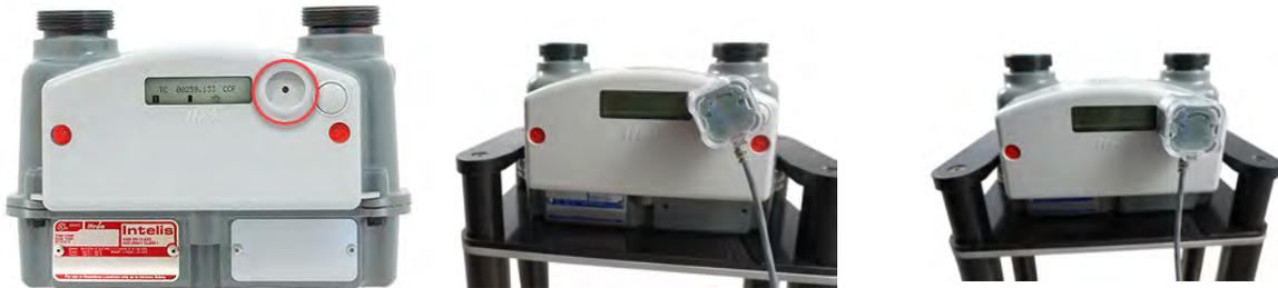
**Note:** The Intelis Gas Meter will automatically go into Test Mode (Menu 6) when the pulse prover output cable is connected.
