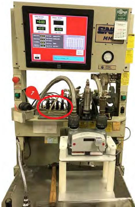
11. Connect the Intelis Gas Meter end of the SNAP pulse prover cable to the Intelis Gas Meter optical port by firmly pressing the aluminum round threads of the cable into the port. Begin by positioning the cable at the 4:30 o'clock position. Tighten the cable to the 6:30 o'clock position.
