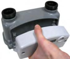
5. Align the new index's screw holes with the screw holes of the meter (oriented as shown in the following image). Slowly align the new index with the meter until it contacts the meter. Gently push the new index onto the meter so that the 6-pin connectors from the meter and the new index fully engage. The new index should be flush with the meter.
