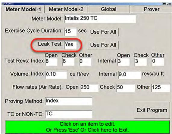
12. Verify or enter **Test Revs: Index Open, Check, Other** settings. Itron recommended settings are listed.
