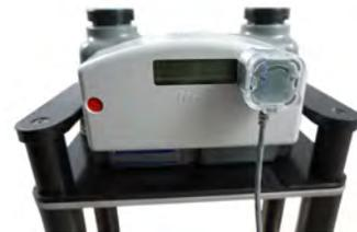
3. Press the EEI prover's green button to begin the proving test.
