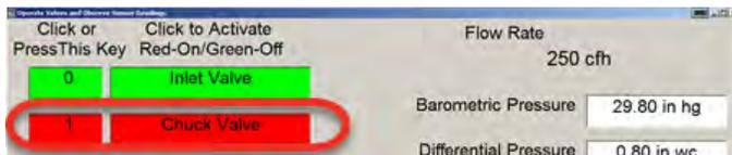
5. After the Intelis Gas Meter is clamped to the prover, turn on the appropriate nozzle in the center of the screen to exercise the meter.
