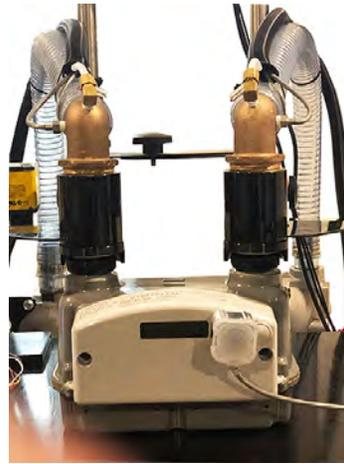
2. Connect the Intelis Gas Meter end of the EEI pulse prover cable to the Intelis Gas Meter by firmly pressing the aluminum round threads of the cable into the port. Begin by positioning the cable at the 4:30 o'clock position. Tighten the cable to the 6:30 o'clock position.
