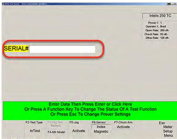
4. Press or click the green bar on the bottom of the screen to begin the Measurement Systems proving test.
