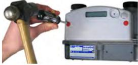
3. There are two screws holding the original index onto the meter located behind the tamper seals just removed. Unscrew both screws while holding the original index. Do not discard the screws.
